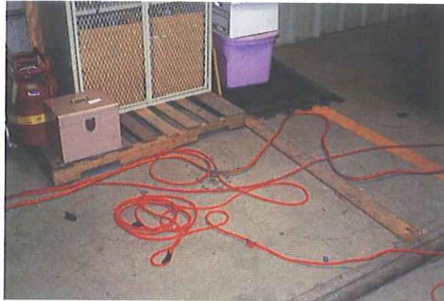
Materials and tools in the walkway
