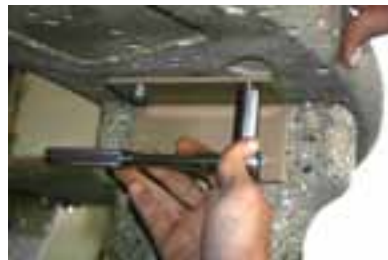
Step 18 Thread all bolts into inserts. Begin tightening until snug. DO NOT OVER TIGHTEN
