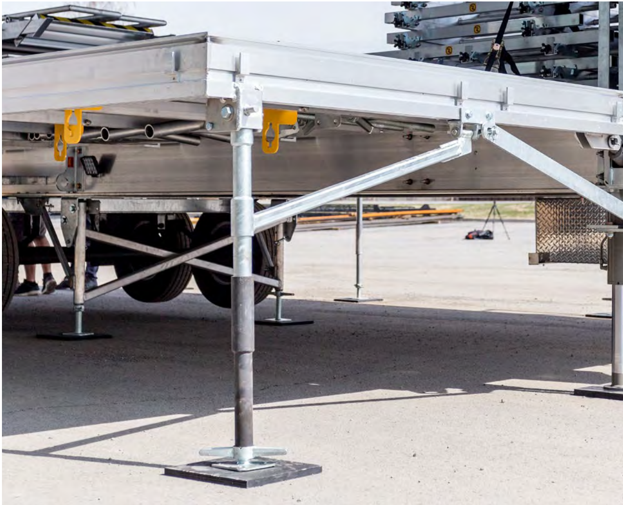
Deck & chassis at 150 lb/ft 2 (732 kg/m 2 ) meets IBC & NBC standards Cross braced steel members added to support legs under the mid-section of trailer frame.
